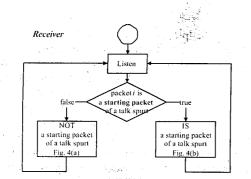
Fig. 3 packet processing flow chart at the receiving end
